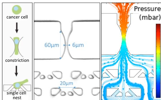
**Fig.1:** Principle of microfluidic device
