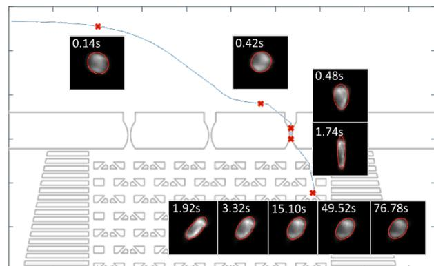
**Fig.2:** Shape evolution of the cell as it crosses the constriction and recovers in the trap
